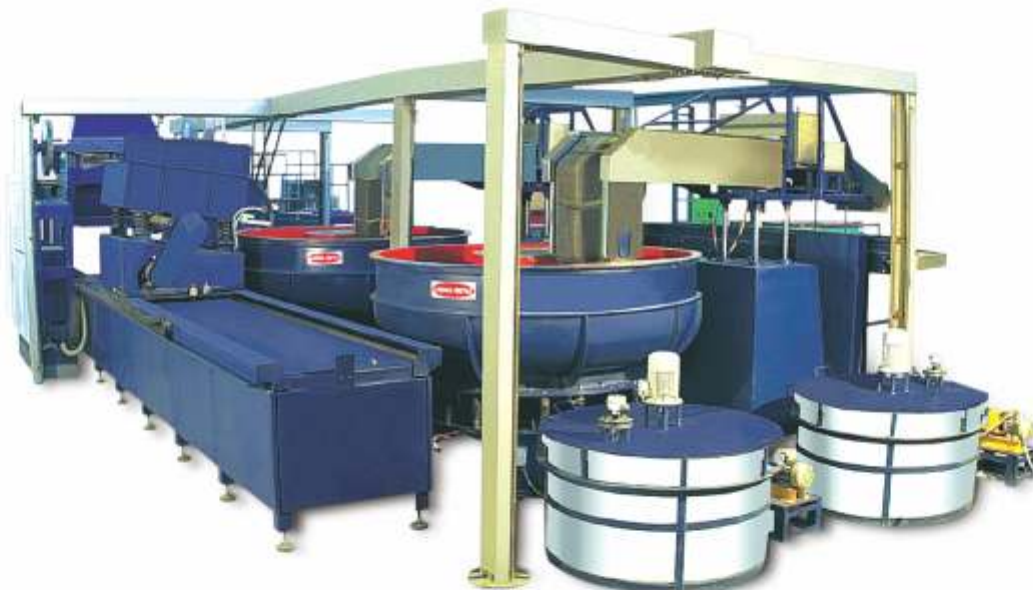
Auto Loading, Vibratory Deburring, Washing & Drying
